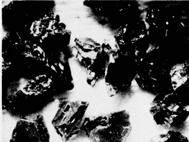
Figure 15. SiC Particles Used for Eroding MgF 2 Magnification: 14X
