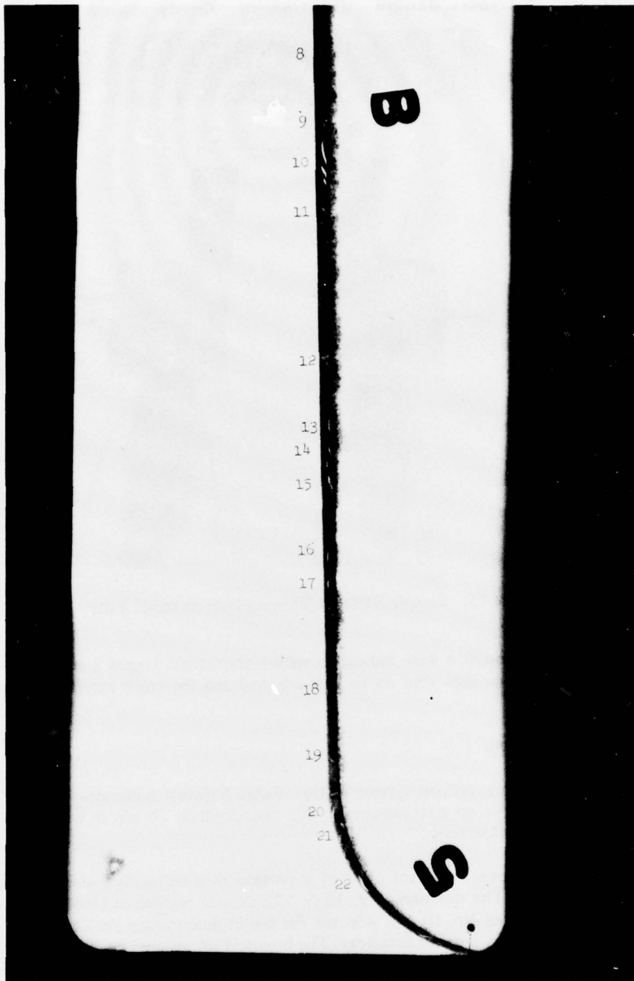
Figure 16. Radiograph of Edgesal with Numerous Voids
