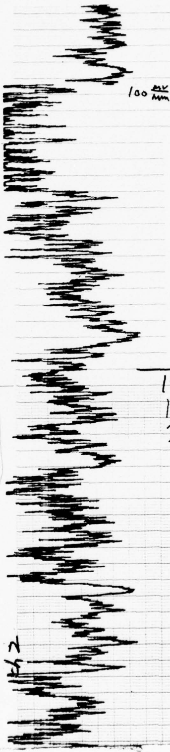
FIGURE 17, Ramble Sensor #1 23 February 1976 - Sample #30 Chart speed .5 cm/min Response to invisible oil film
