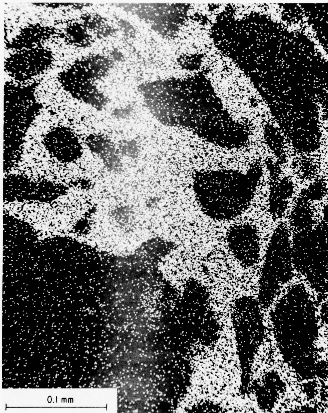
Figure 20. Scanning electron micrograph formed by using excited silicon X-ray emission intensity of modulate cathode ray tube image. (Same area as in Figure 19b.) Dark regions are epoxy, light regions are char.
