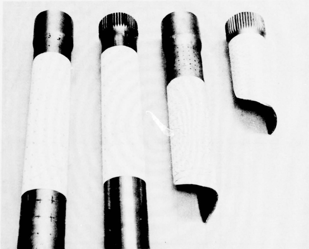
Figure 17 - Torsion tubes with their associated isostress patterns attached. The two tubes on the left survived fatigue test and display much more uniform isostress patterns than the two tubes on the right, both of which failed fatigue test.
