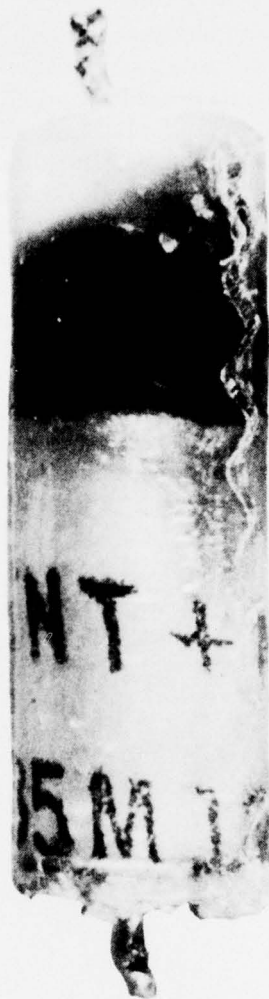
Figure 1. A TNT356U012P18 capacitor which will fail soon. The black in the top portion is electrolyte leaking out of the primary section.
