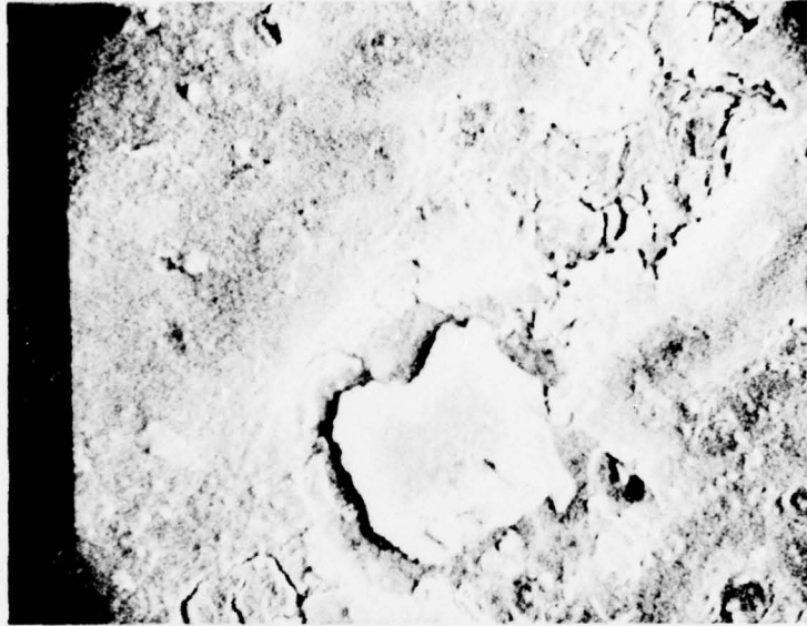
Figure 13. Pitting at Inclusions (30 Knots: -1.0 V_{Ag/AgCl} )
