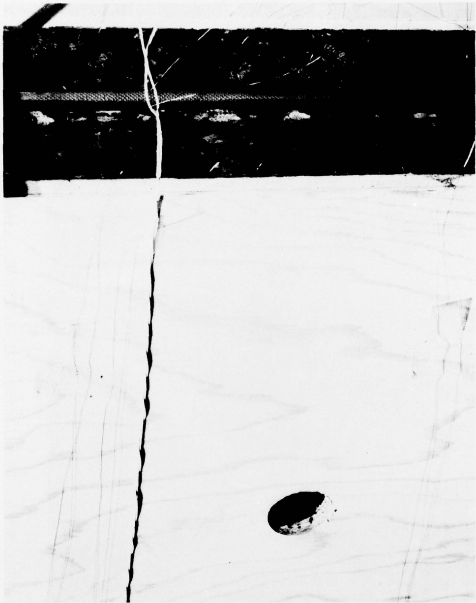
Figure 6. Close-up view of an unplugged surface thermocouple hole and the ends of the two cork boards.
