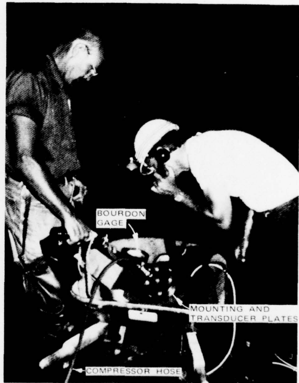
Figure A1. Field calibration check of pressure transducer
