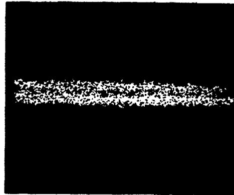
b. Final adjustment (dark band between noise bands has just vanished).
