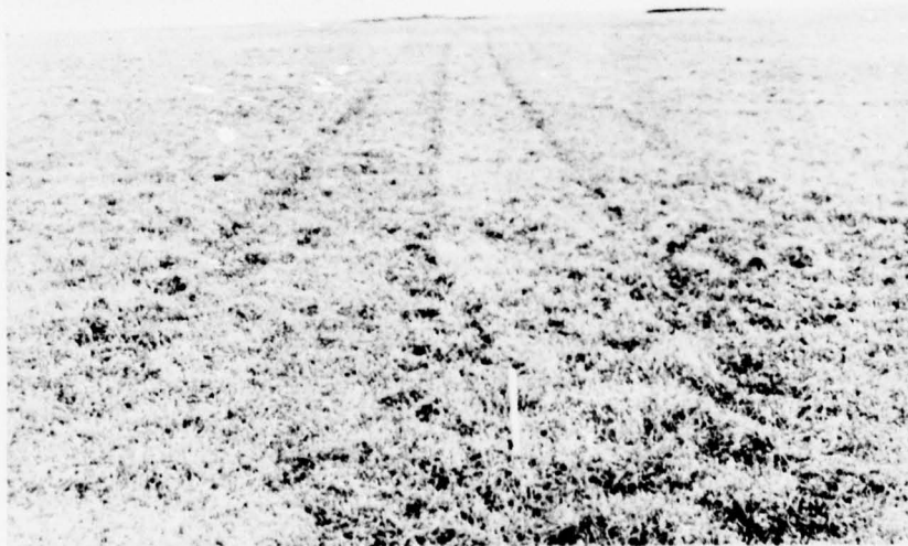
Figure 11. Rolligon impact in Type U3 after a single pass.
