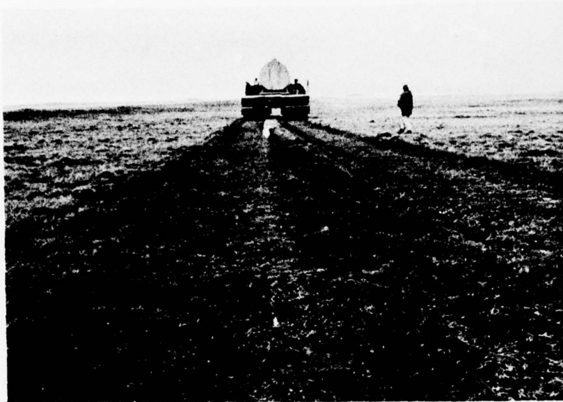
Figure 19. Multiple Pass Test Lane No. 2 immediately after 30 passes. Vegetation is Type U3.
