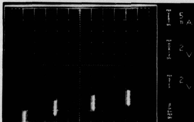
Leakage in Logic TFT V_{GS} = -10V
