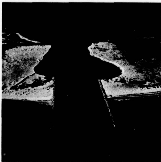
Figure 2.59 Erosion Has Widened the Bob Sikes Channel, St. George Island.
