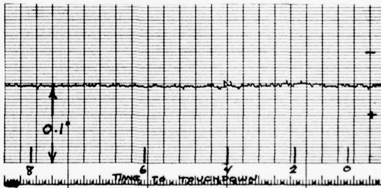
Figure 5-18 FLARE SCENARIO - SEP RECEIVER (DELAY & COMPARE) 8 FT. AIRCRAFT ANTENNA HT., 0 dB MULTIPATH, 30 dB SIDELOBES
