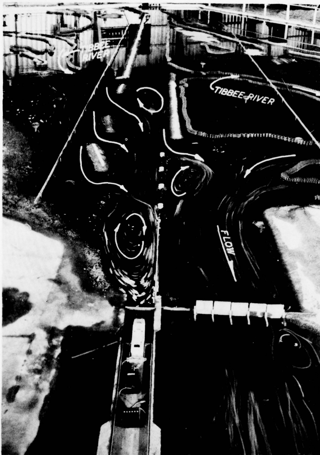
Photo 5. Plan D-2 with discharge 57,000 cfs in Tibbee River and none in Tombigbee River and upper pool elevation of 162.9. Note eddies and intensity of crosscurrents in the lock approach compared with normal distribution of flow (Photo 3)
