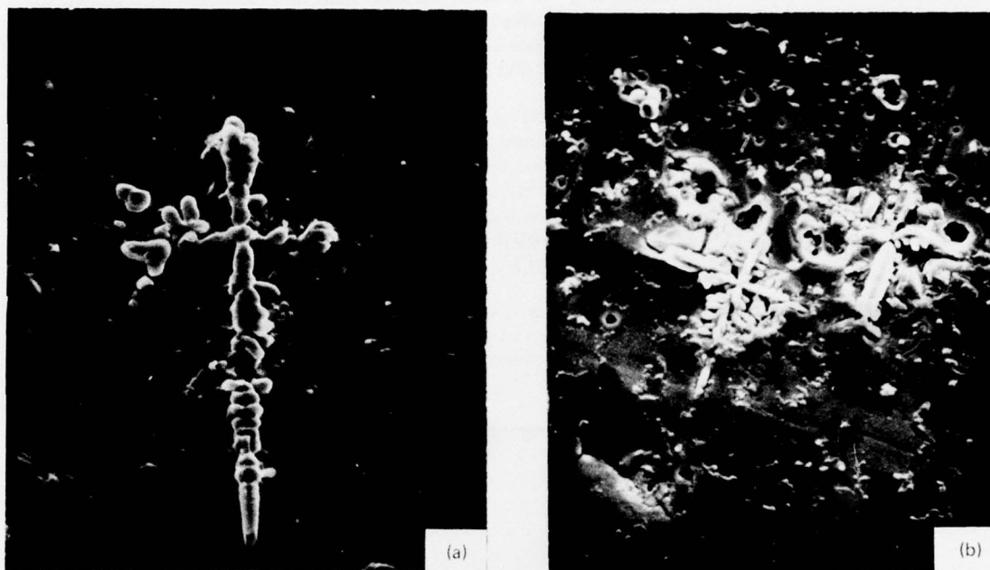
Fig. 6. "Two examples of etched surfaces of Tb_{0.3}Dy_{0.7}Fe_2 showing the three pseudobinary phases. Bright cross-like structures in sharp relief are (Tb, Dy) oxide or nitride. Slightly etched needle-shaped depressions are (TbDy)Fe_3 . Major smooth surface is (Tb, Dy)Fe_2 , the desired Laves phase.
