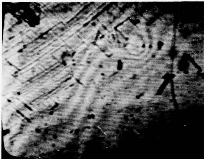
Fig. 6. An example of a Widmanstätten precipitate is shown in the upper left corner. It has a cross-hatched pattern with regular angles. The stripes are about 1 \mu\text{m} wide.
