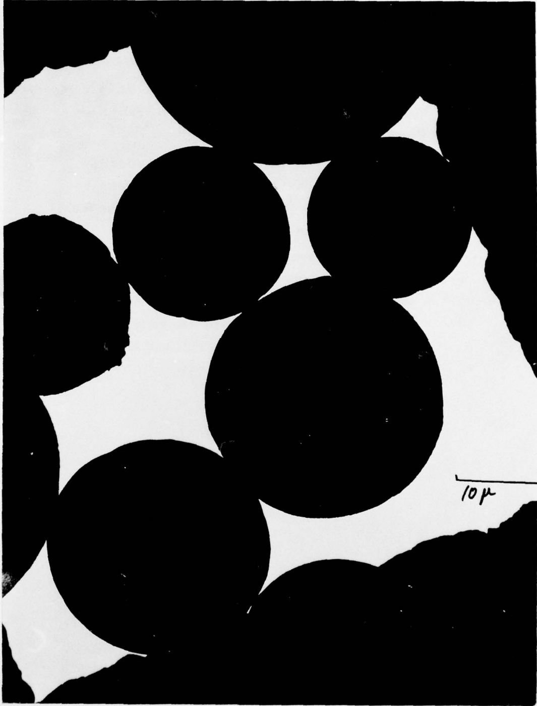
Figure IV-23. Aluminum oxide particles that have been spherulitized by melting powders in a plasma spray.
