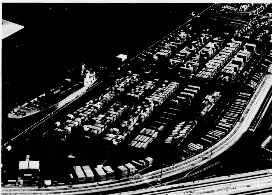
This 35-acre container terminal at the Port of Los Angeles features a 40-ton crane that can load two containers simultaneously in about 3 minutes. (Photo courtesy of Port of Los Angeles)
