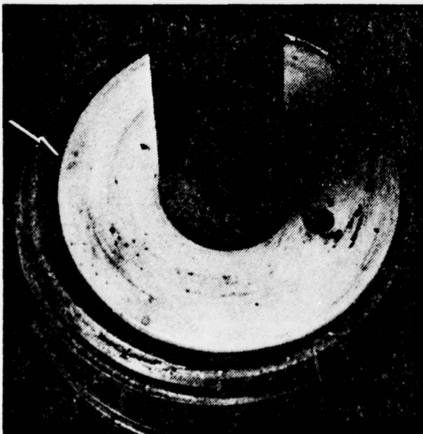
Figure 6. Extruded Seal, Main Cable Seal (Approx. life size)
