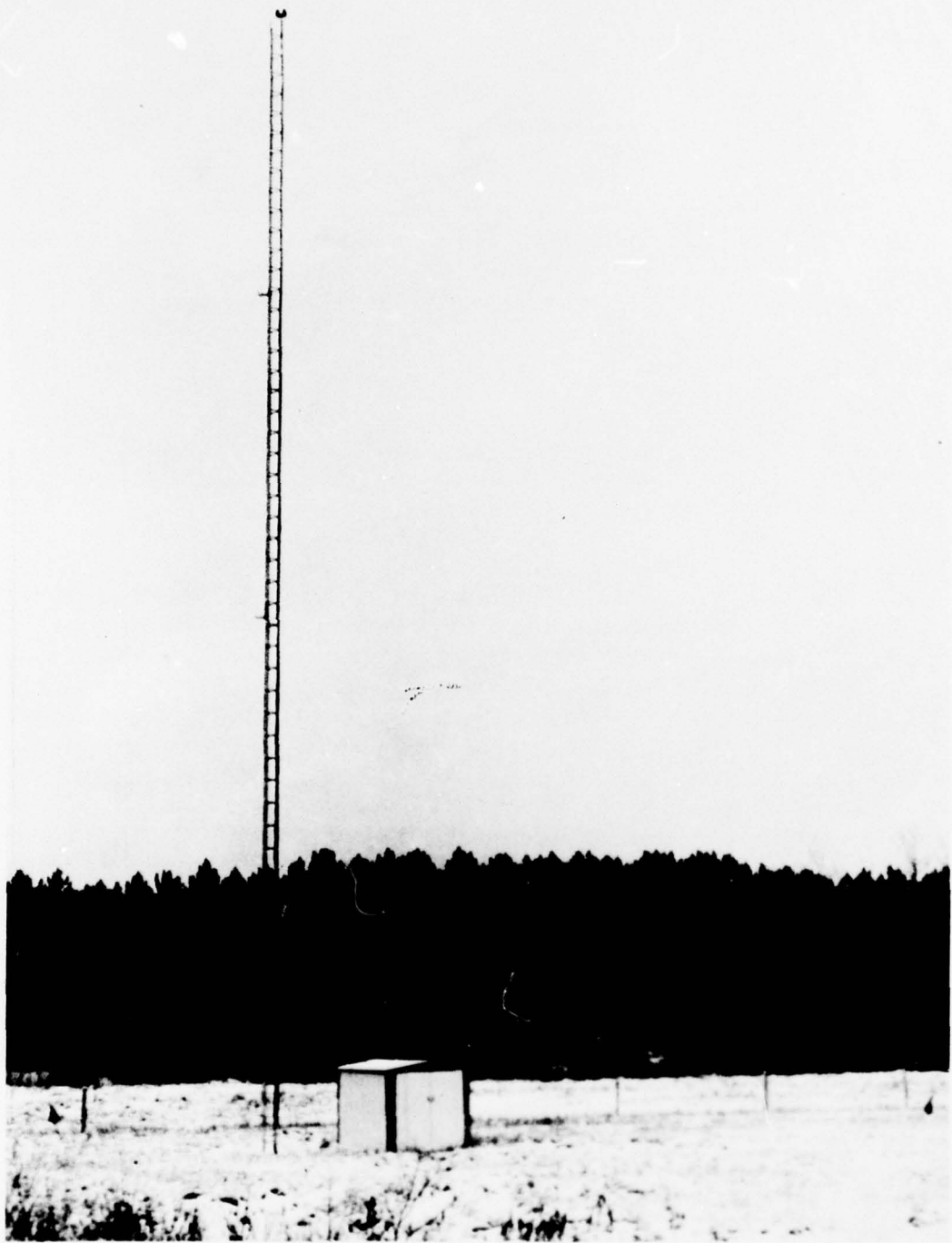
Figure 2. Gradient Clearance Far-Field Monitoring Probes Used by Ohio University at the Michigan Snow Site.
