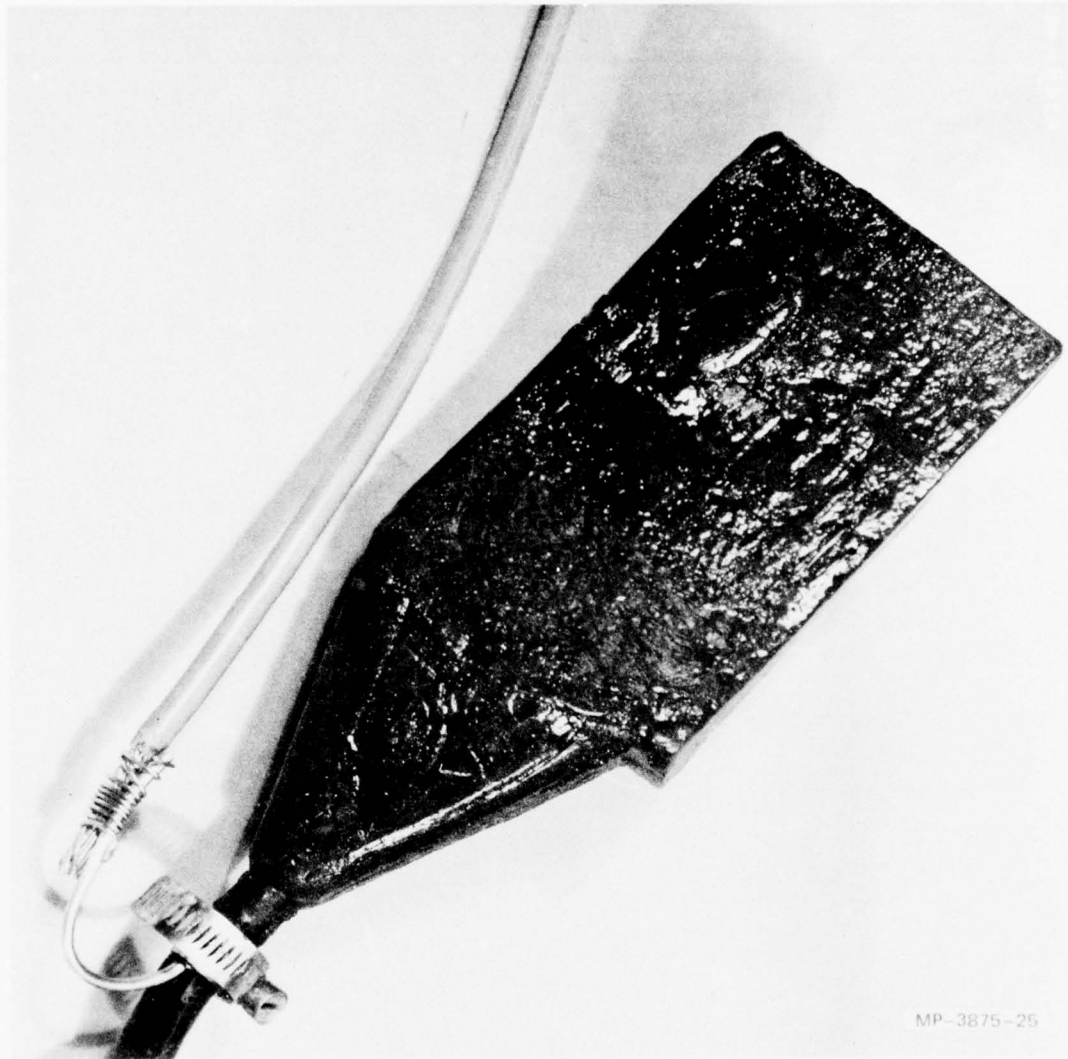
FIGURE 5 COMPLETED PADDLE GAGE ASSEMBLY (COURTESY OF WATERWAYS EXPERIMENT STATION)
