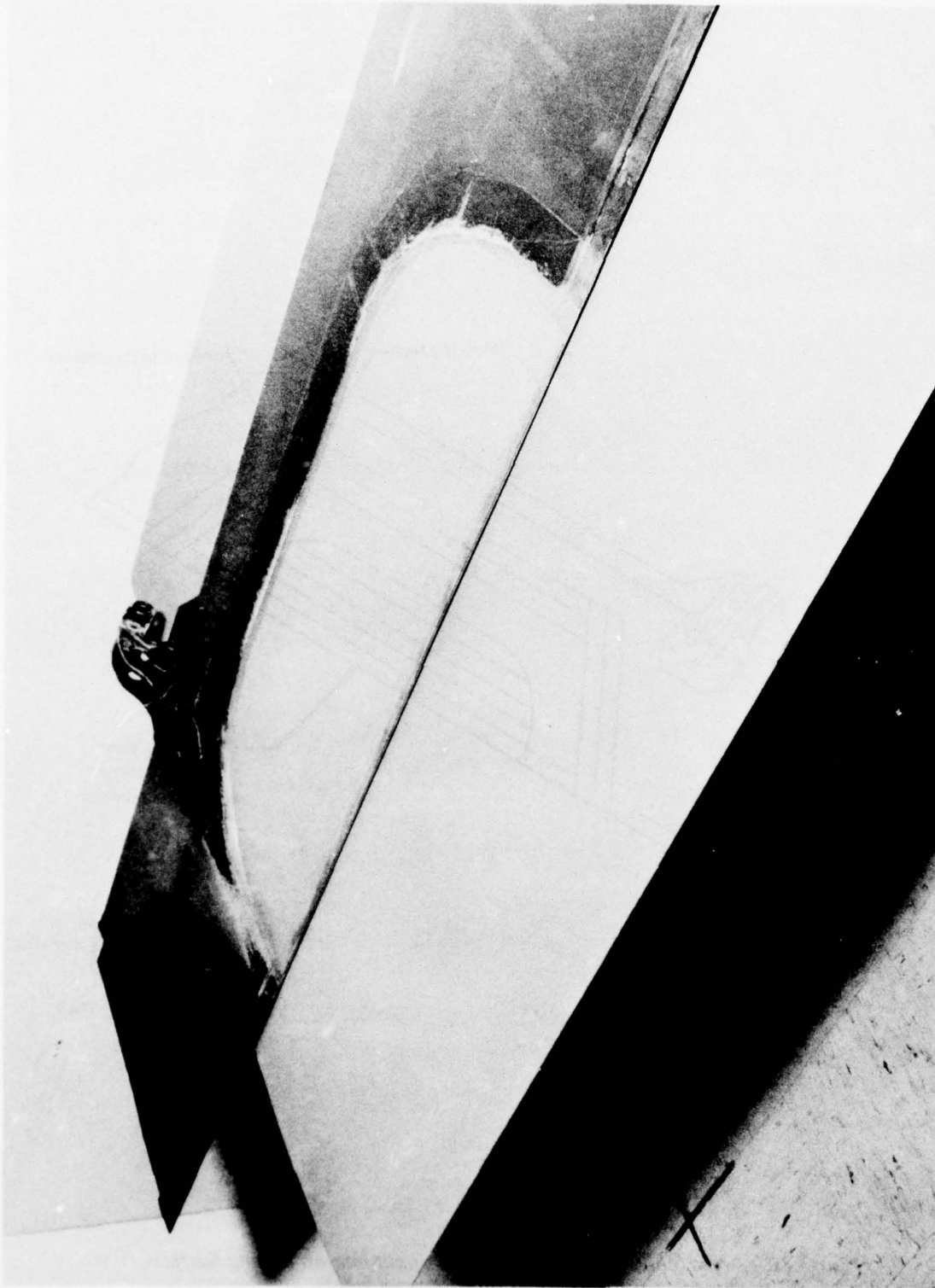
Figure 20.—Nonflush Patch on the Lower Surface
