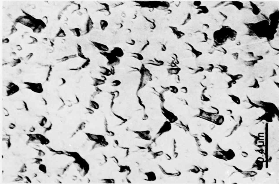
c d Figure 4. Transmission Electron Micrographs: c) Surface of Film Generated by 60V, 1.0M, 5-Second Anodization; d) Surface of Film Generated by 60V, 1.0M, 300-Second Anodization.
