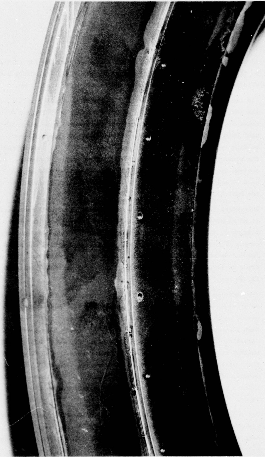
Fig. 10 Close-up View of Inconel Wire Tack-Weld
