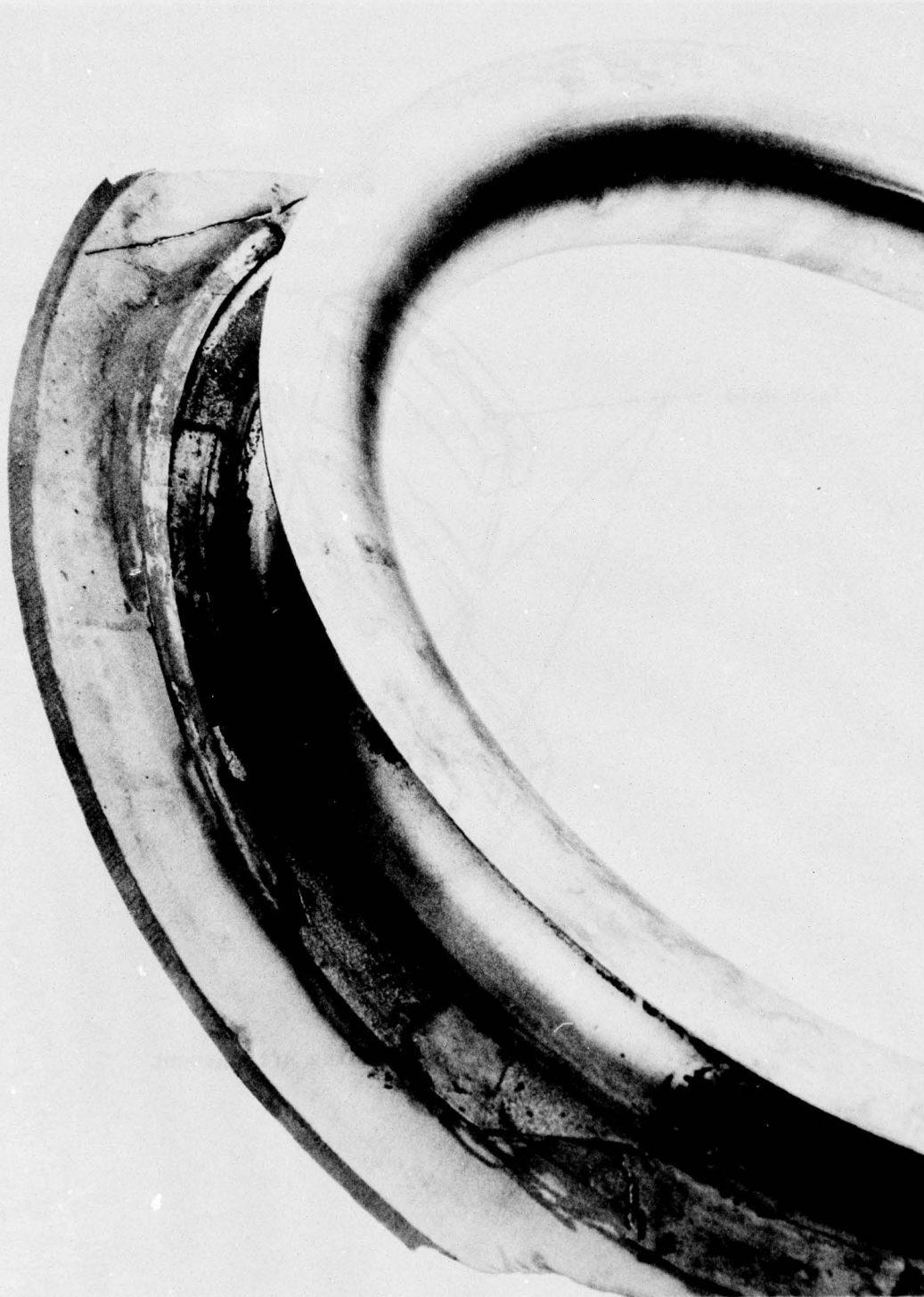
Fig. 8 "Seal No. 3 - Effects of Silver Braze Alloy on Inconel" (Note severe stress corrosion cracking)
