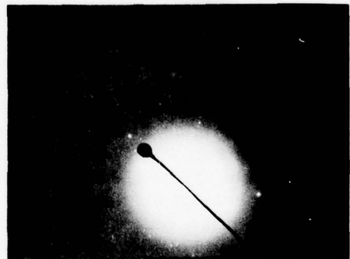
Figure 5. Same as Figure 3 Showing Highly Amorphous Ring Structure.
