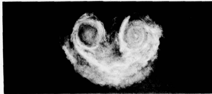
FIGURE 3-5. DEVELOPMENT OF VORTEX INSTABILITY IN WATER TANK TESTS
