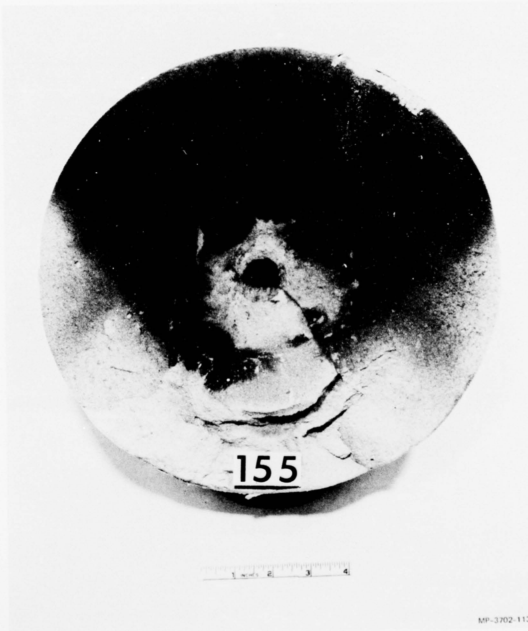
FIGURE 50 HYDROFRACTURE FROM AN EXPLODED CAVITY - TEST 155
