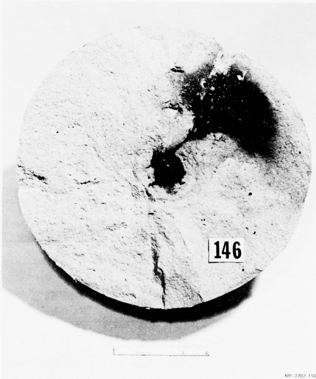
FIGURE 48 HYDROFRACTURE FROM AN EXPLODED CAVITY – TEST 146 (Concluded)
