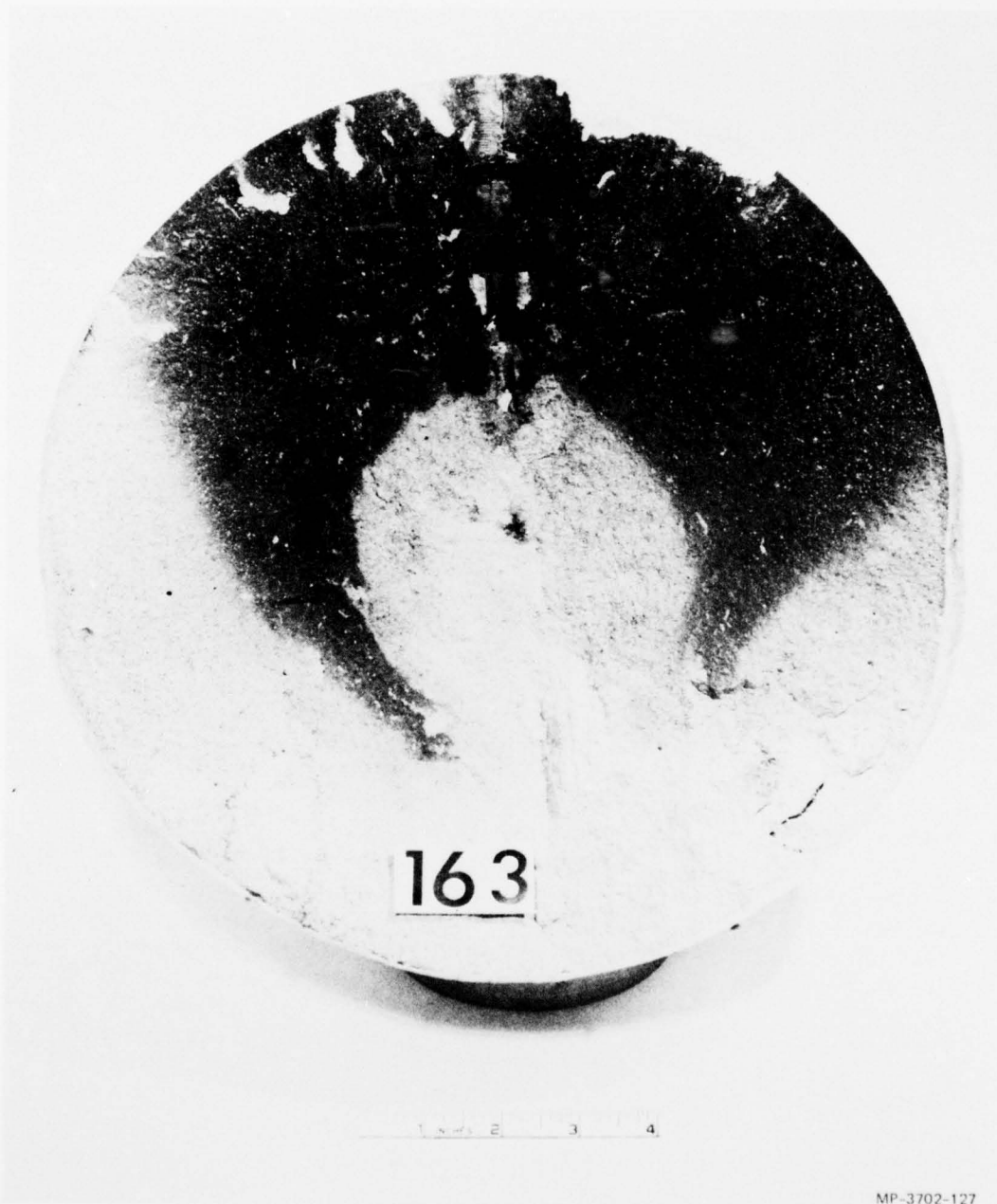
FIGURE 52 HYDROFRACTURE FROM LOCALITY AWAY FROM AN EXPLODED CAVITY — TEST 163
