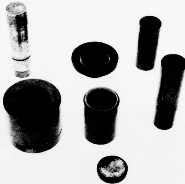
FIG. 1 - Tool steel die used to prepare the briquetted specimens.
