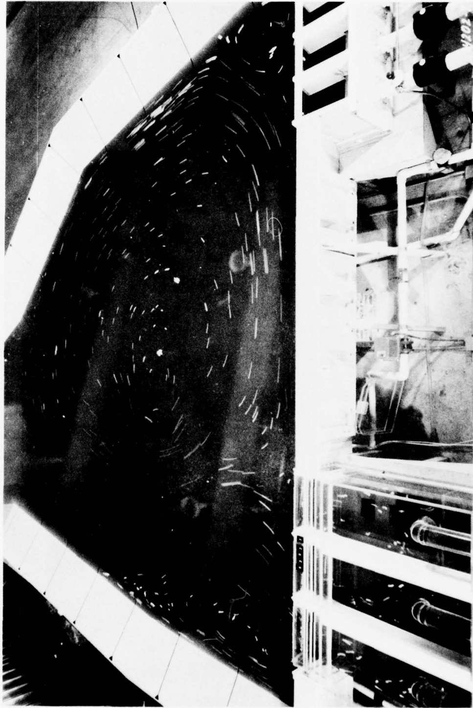
a. Proposed station operating independently Photo 1. Flow patterns in approach channel (original design); sump el 228 (sheet 1 of 2)
