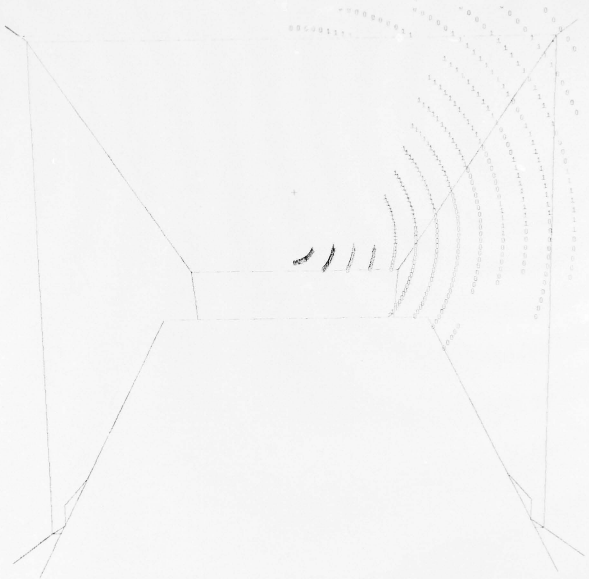
Figure 4. Primary reflection points on the right-hand side of the canopy and their associated reflectance values.
