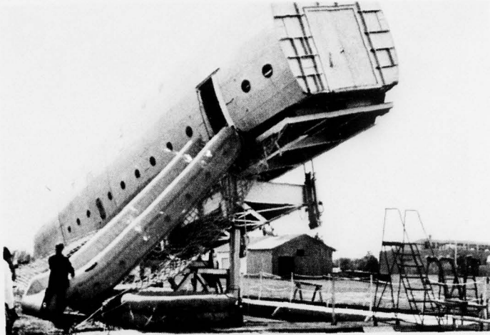
Figure 2. The evacuation simulator positioned 12^{\circ} nose down and in a 12^{\circ} left roll as in an emergency landing with nose gear and left main gear failure.
