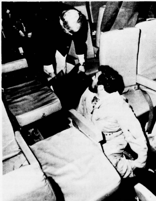
Figure 7. A paraplegic test subject being assisted down the aisle with the aid of a blanket.
