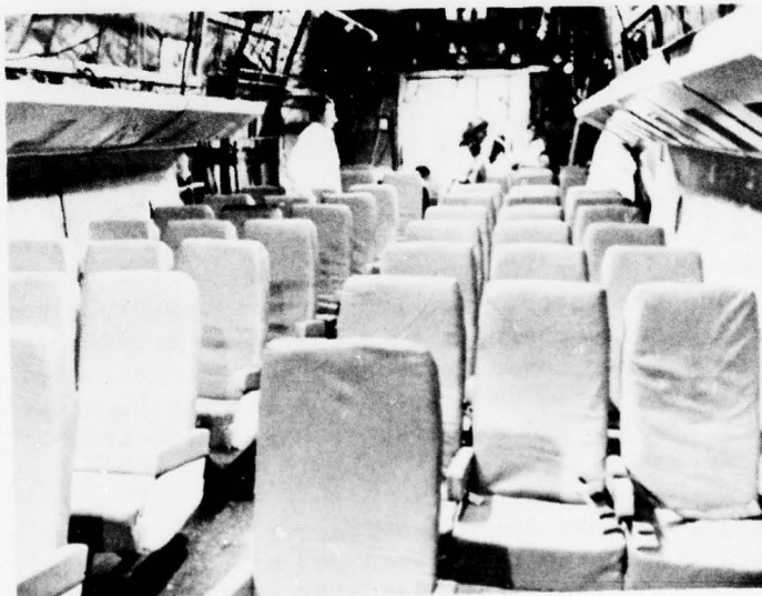
Figure 3. Seating configuration of the evacuation simulator.
