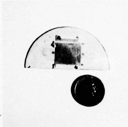
Fig. 2.4.8a. The Sensor (CdS, contacts, transducers, on \text{LiNbO}_3 ). Note the size relation to a U.S. one cent piece.
