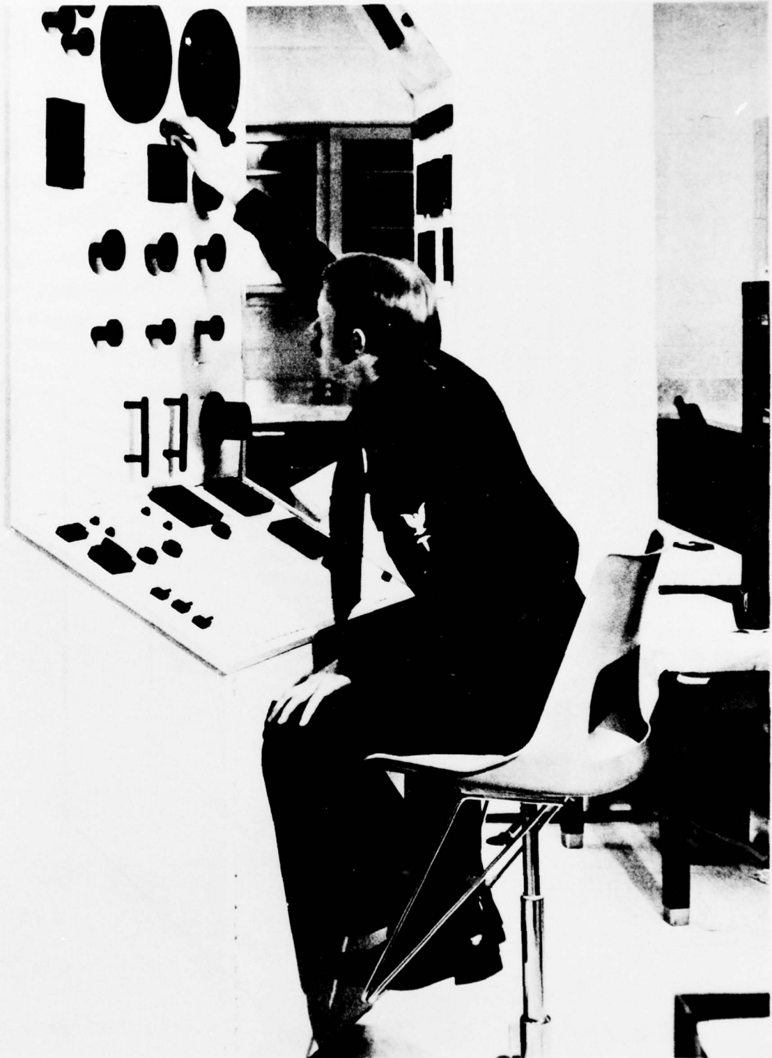
Fig. 21. A seated diver able to reach selected control panel #3007875 because his seat has been raised 11 inches.
