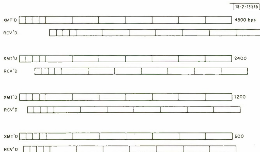
Fig. 4. Effect of round trip propagation delay on frame-by-frame basis relative to the bit rate of a satellite channel.
