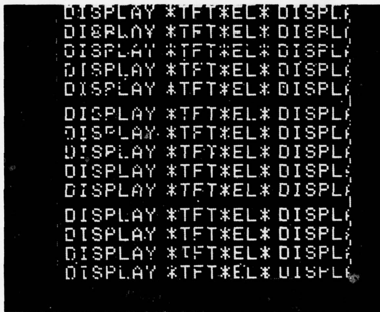
Fig. 2. Improved Level of Operation in 6" x 6", 30 lpi 2 Level Electroded TFT-EL Display
