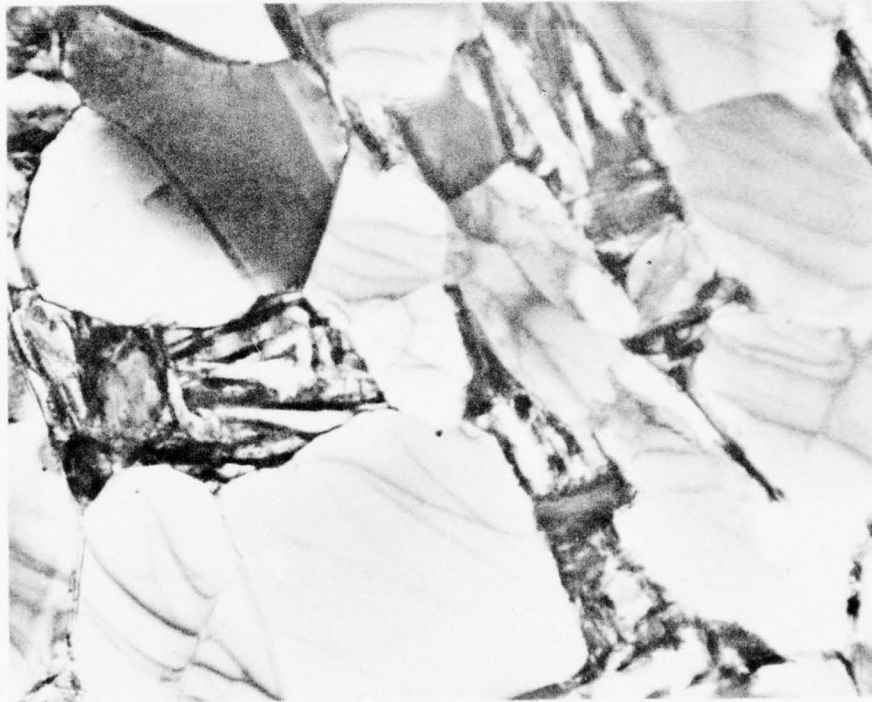
Figure 19. Transmission electron micrographs showing equiaxed alpha and transformed beta in alpha-beta annealed (a) Ti-6Al-4V-0.05Y and (b) Ti-6Al-4V-0.080MM.
