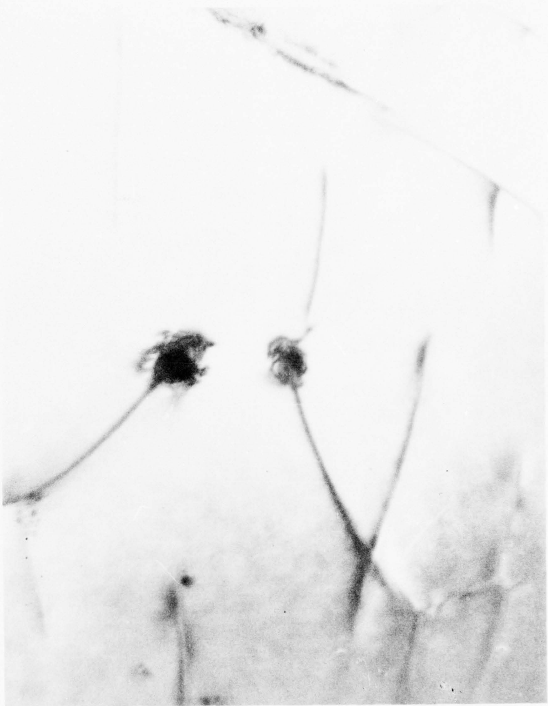
Figure 41. Formation of Orowan and prismatic loops at dispersoids during the initial deformation of Ti-6Al-4V.
