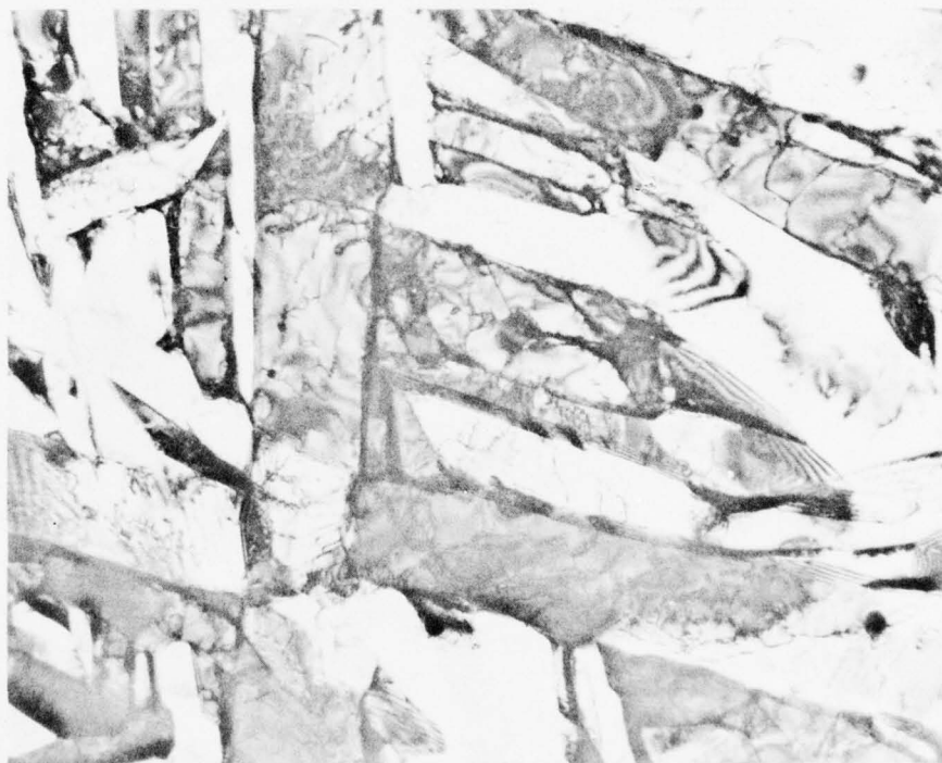
Figure 17. Transmission electron micrographs of beta-annealed (a) Ti-6Al-4V reference alloy and (b) Ti-6Al-4V-0.050Y.
