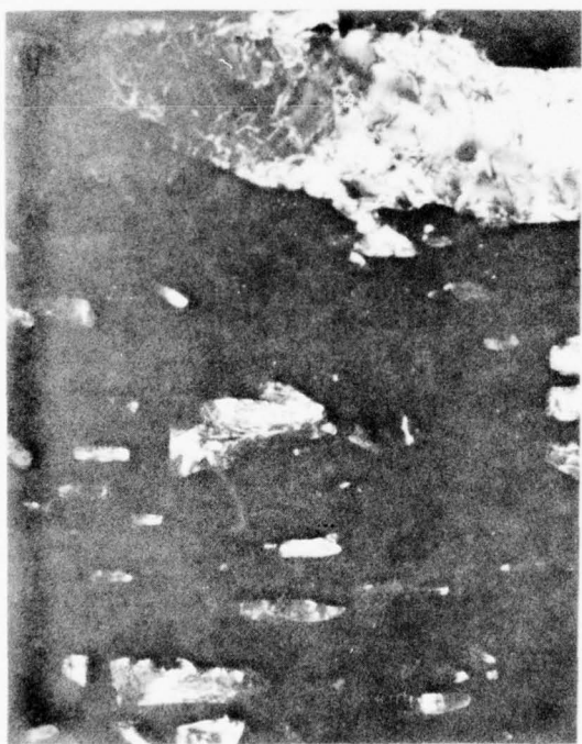
Figure 29. Dark-field electron micrograph of beta precipitates in alpha-prime phase of Ti-6Al-4V reference alloy quenched from 1020°C and aged for 24 h at 550°C.
