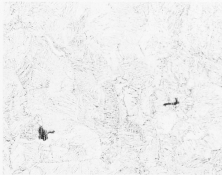
Figure 30. Microstructures of beta-annealed and air-cooled (a) Ti-6Al-4V reference alloy and (b) Ti-6Al-4V-0.05Y (heat treatment C, Figure 14).
