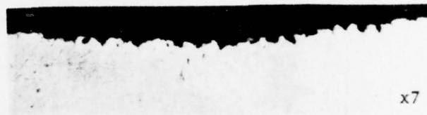
(B) LONGITUDINAL CROSS SECTION SHOWING PROFILE OF THE FORWARD ERODED GROOVE
