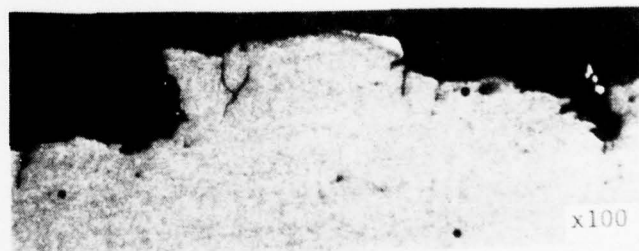
(D) MICROSCOPIC SURFACE VIEW OF THE FORWARD GROOVE SHOWING SEVERAL CRACKS
