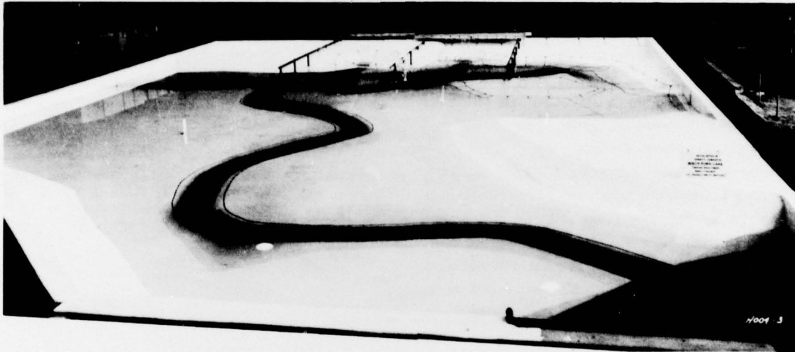
Fig. 2. 1:36-scale model of Beech Fork Reservoir and Outlet Works
