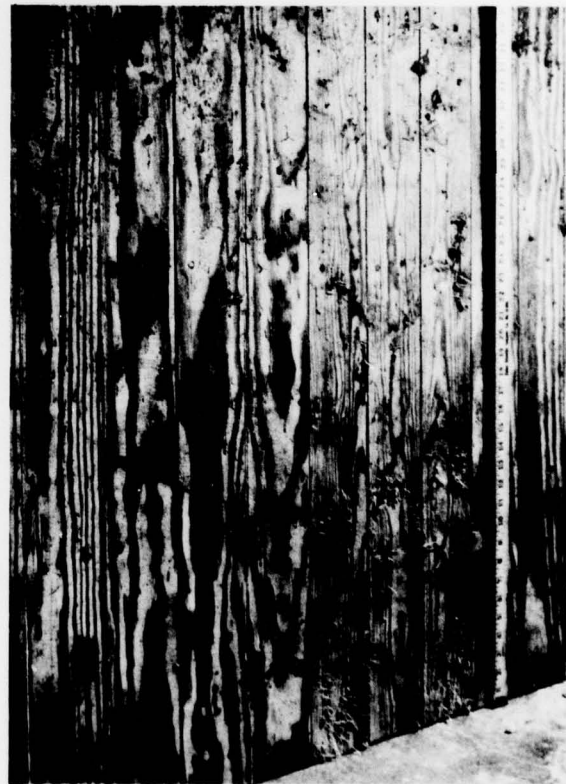
Fig. 2. Block 1, detail of side A showing abrasive action on wood
