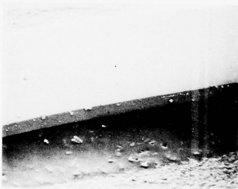
Figure 9. Side of Bonded Silicon Gage (650X)
