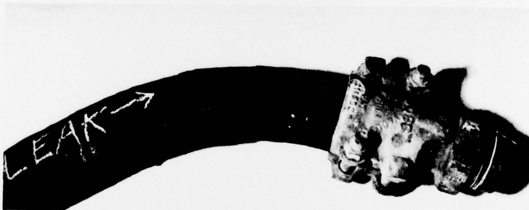
Figure B-2. Cover damage on 2-inch stainless steel-lined rubber hose caused by sharp 90-degree bend at ship's intake.
