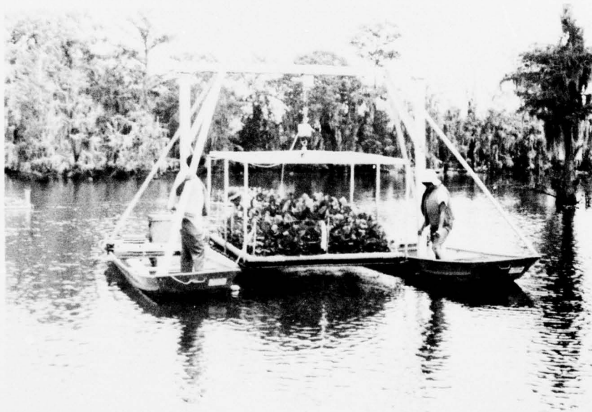
Figure A3. Weighing apparatus in operation, with the test plot suspended through the load cell
