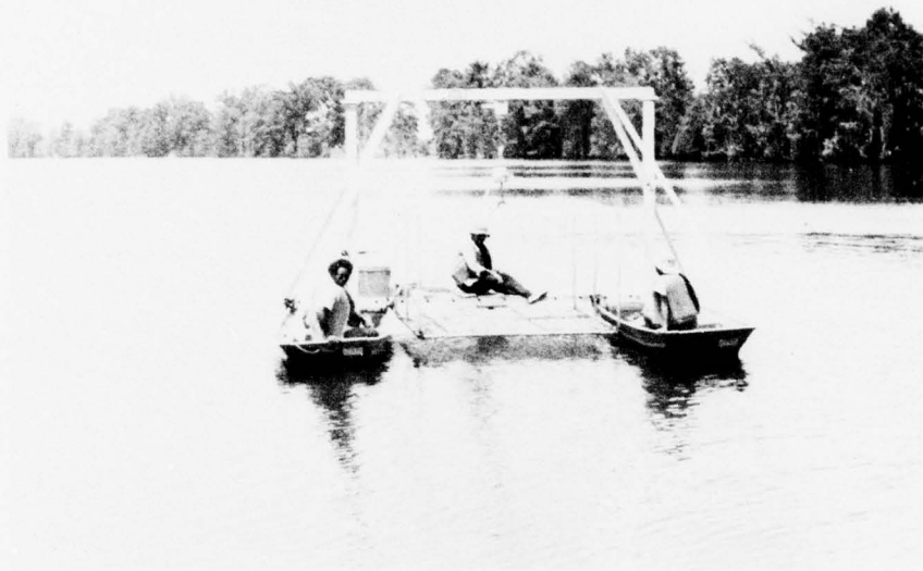
Figure A2. General view of the weighing apparatus used to weigh the frames (Figure A1)
