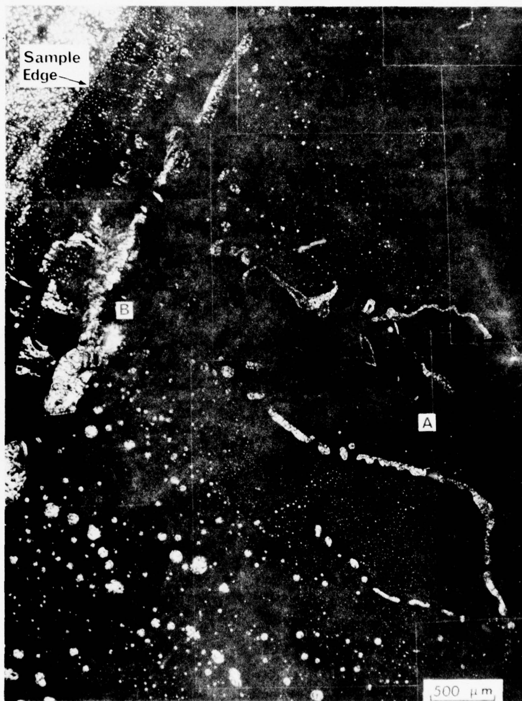
FIG. 55. BANDS OF COALESCED MESOPHASE WHICH FORMED AT THE EDGE OF THE LIQUID SAMPLE DURING HOT STAGE PYROLYSIS OF ACENAPHTHYLENE
