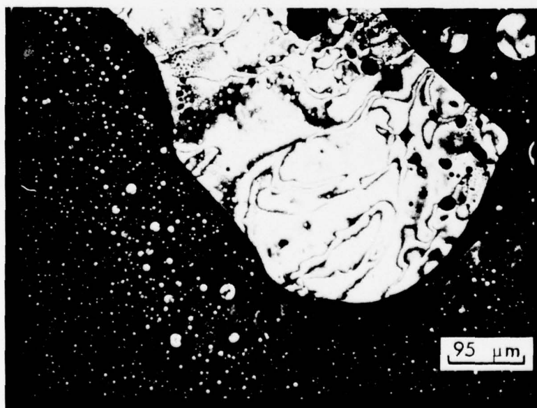
FIG. 61. LARGE DROPLET OF COALESCED MESOPHASE FORMED DURING HOT STAGE PYROLYSIS OF ACENAPHTHYLENE
