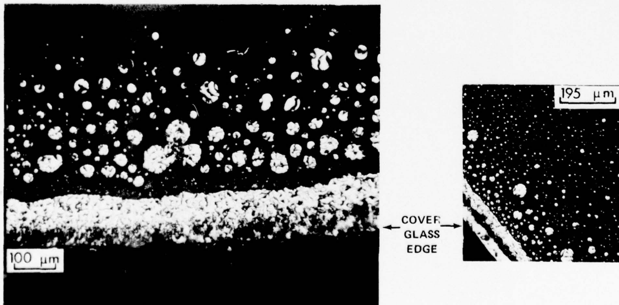
FIG. 55. BANDS OF COALESCED MESOPHASE AT THE EDGE OF THE SAMPLE COVER GLASS
