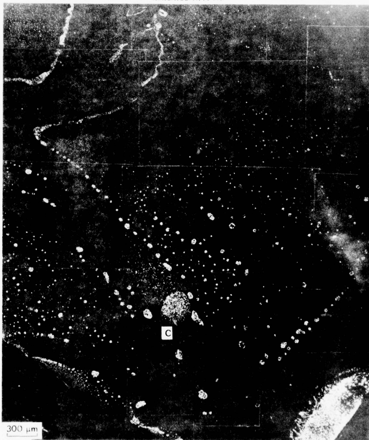
FIG. 50. COMPOSITE PHOTOGRAPH OF MESOPHASE DROPLETS ORDERED DURING PYROLYSIS BY GAS BUBBLE MOVEMENT
