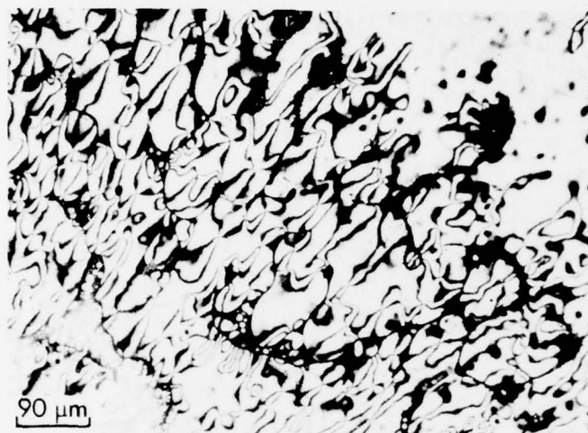
FIG. 60. REGION OF COALESCED MESOPHASE CONTAINING A HIGH CONCENTRATION OF EXTINCTION CROSSES
