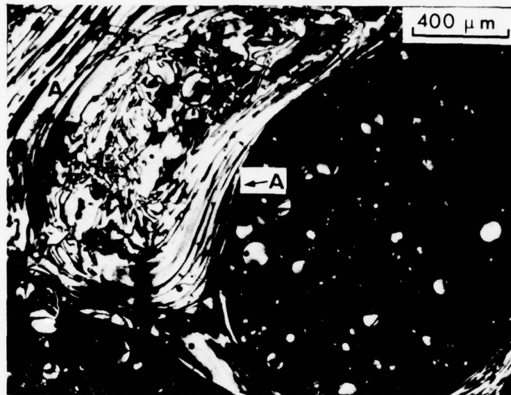
FIG. 23. FIBROUS MICROSTRUCTURE IN THE COALESCED MESOPHASE FROM ACENAPHTHYLENE
