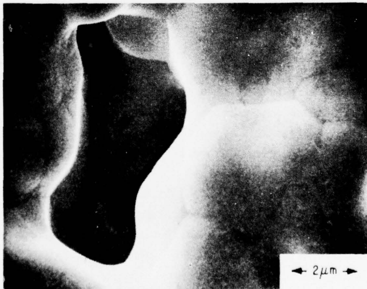
Figure 19. SEM of MK-2 Au powder with 10 vol pct of E1527 glass removed after sintering at 800°C for 600 s.
