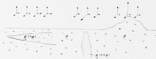
b. Major VLF field changes known to take place when local changes in earth conditions are encountered.
