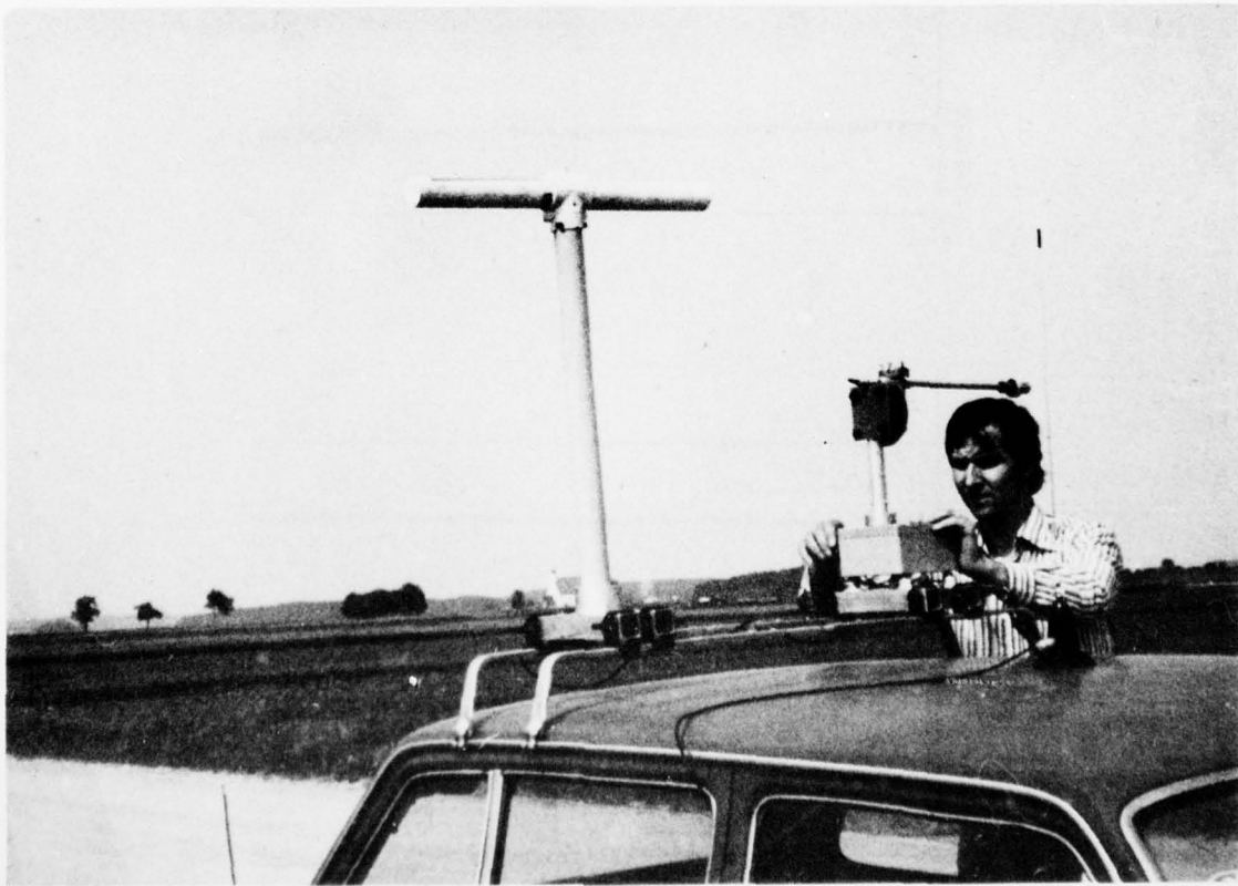
Fig. 6 Vehicle transmission unit with horizontal polarized antennas on top of a car
