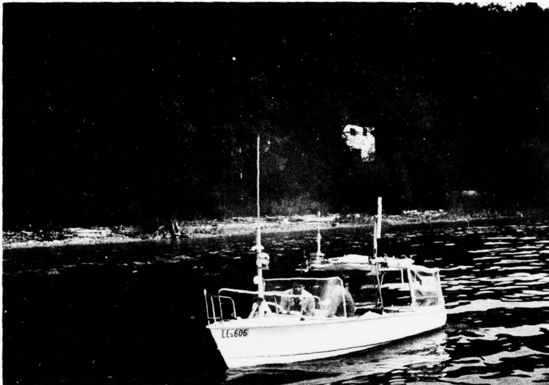
Fig. 7 Vehicle transmission unit with vertical polarized antennas on a motor-boat.
