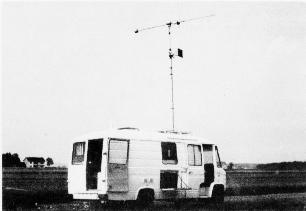
Fig. 8 Fixed station vehicle with medium gain receiving antennas.
