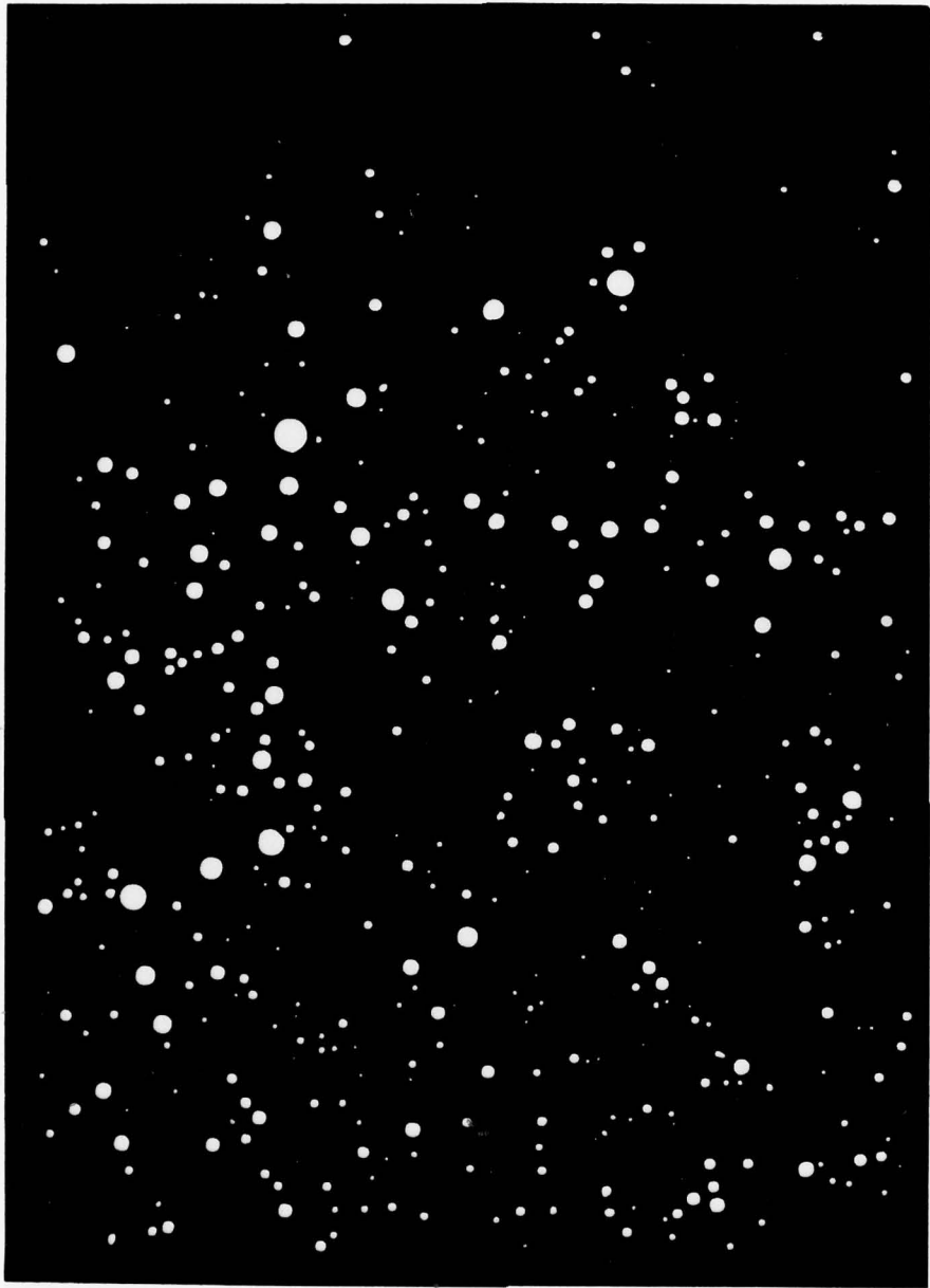
Figure 6-6 Typical Magnified Photograph of Water Droplets on Greased-Slide (Relatively Small Diameters)
