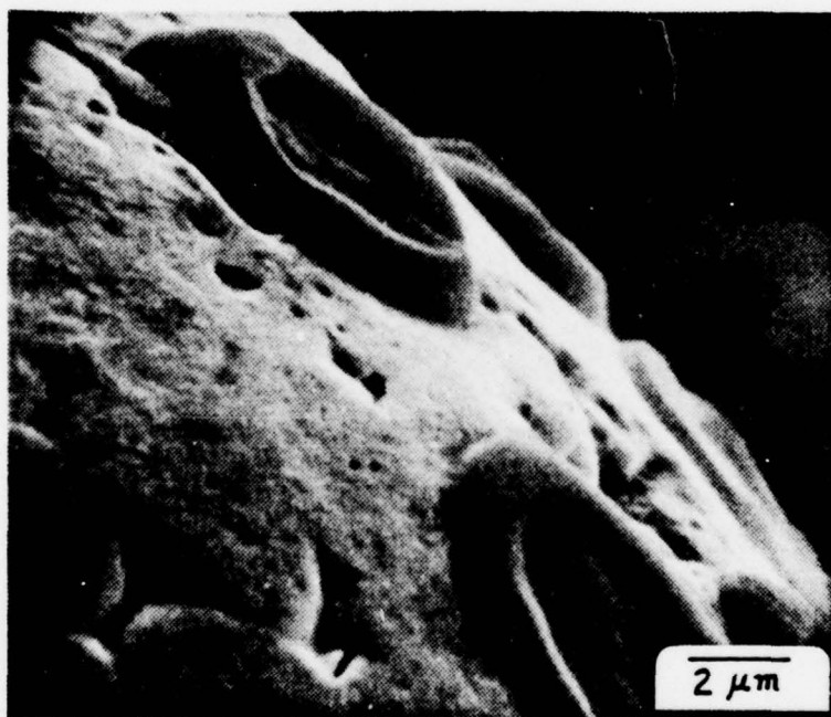
Figure 75. Closeup profile view of "pancake" shaped oxidation products on plated sphere; height of products is clearly visible; 30 seconds at 50 \text{ mA/cm}^2 in 9.96\text{N KOH} , 6300\times .
