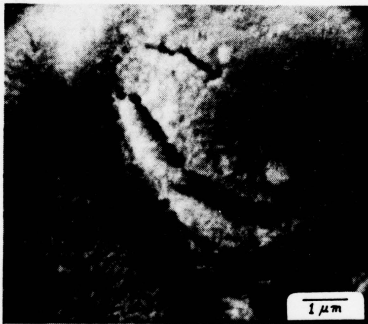
Figure 39. Zinc anode, region B; closeup view of smooth, thick oxidation layer showing surface cracks and "furry" texture; 21 minutes at 1.67 \text{ mA/cm}^2 plus 12 minutes at 6.67 \text{ mA/cm}^2 in 9.96N KOH, 13000X.
