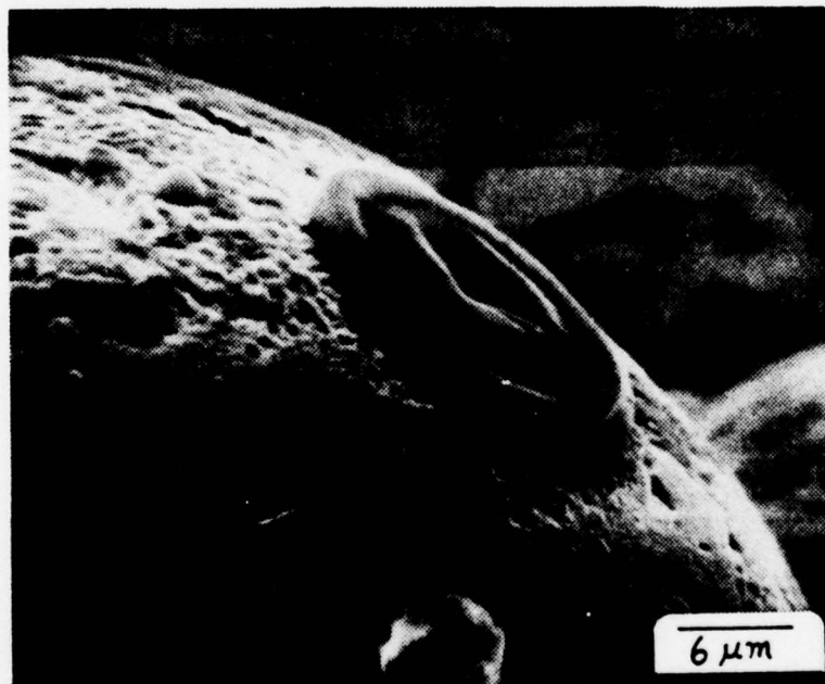
Figure 74. View of single "pancake" shaped oxidation product on plated sphere surface; dimpled center is visible; 30 seconds at 50 \text{ mA/cm}^2 in 9.96N KOH, 2500X.
