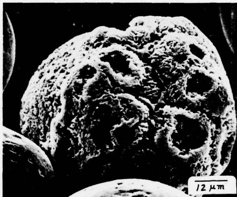
Figure 71. Advanced stage of "salt and pepper" oxidation product growth on plated sphere surface; thick, crusty product has developed; 30 seconds at 10 \text{ mA/cm}^2 in 9.96N KOH, 1250X.
