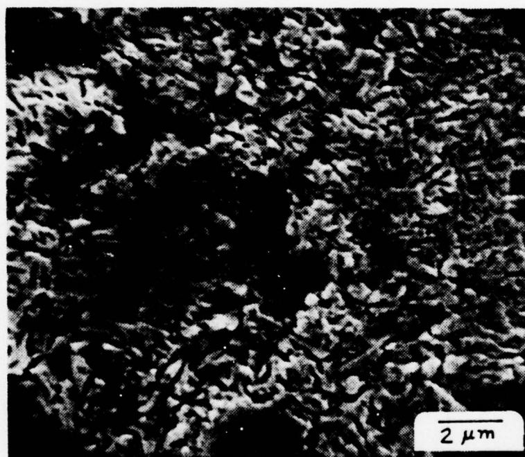
Figure 68. High magnification view of a dense "salt and pepper" oxidation product layer on a plated sphere surface; individual constituent white and gray products are distinguishable; 30 seconds at 25 \text{ mA/cm}^2 in 9.96N KOH, 6300X.
