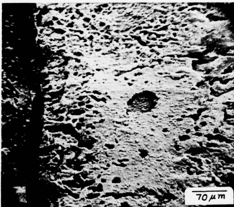
Figure 23. Zinc anode, region A, next to separator; heavy oxidation product layer covering pitted surface; 21 minutes at 1.67 \text{ mA/cm}^2 plus 12 minutes at 6.67 \text{ mA/cm}^2 in 9.96\text{N KOH} , 220X.
