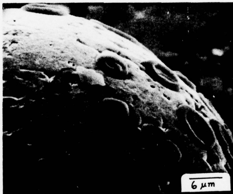
Figure 73. Profile of "pancake" shaped oxidation products on plated sphere surface; 30 seconds at 50 mA/cm 2 in 9.96N KOH, 2500X.
