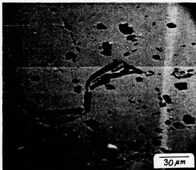
Figure 20. Zinc anode, region A, 0.25 mm from separator; local large pits and possible grain boundary etching; 10 minutes at 1.67 \text{ mA/cm}^2 in 9.96N KOH, 520X.
