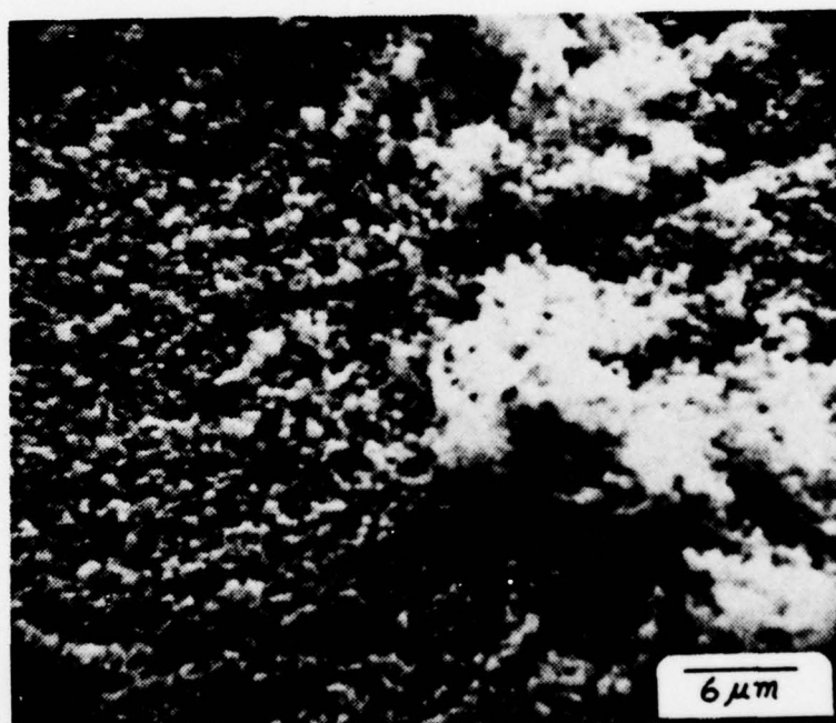
Figure 49. Zinc anode, region B; gray and white oxidation products, white product showing vertical growth; 15 minutes at 10 \text{ mA/cm}^2 in 9.96\text{N KOH} , 2400\times .
