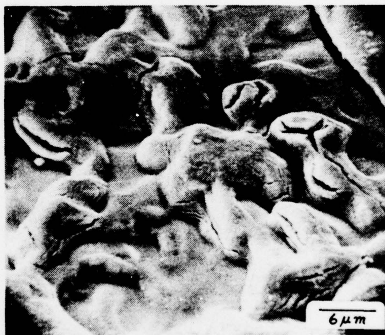
Figure 38. Zinc anode, region B; cumulative buildup of oxidation products resulting in smooth, rounded surface; 21 minutes at 1.67 \text{ mA/cm}^2 plus 12 minutes at 6.67 \text{ mA/cm}^2 in 9.96\text{N KOH} , 2600\times .
