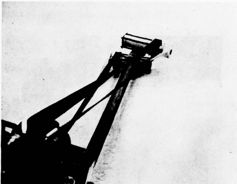
Photo 8 - Power Transmission System Note 90° twist of belts. Belt on right side is twisted clockwise; belt on left side counter- clockwise
