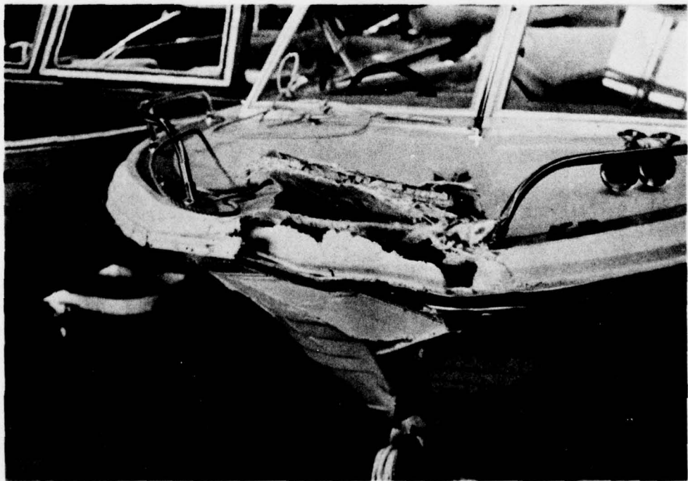
FIGURE 4. STRUCTURAL DAMAGE TO BOW
